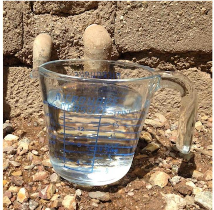
Using a measuring cup and a watch, this AC unit was determined to yield about 2 cups of water every five minutes on a humid August day. This equals around 36 gallons every 24 hours in these conditions. This amount would drop to zero on a cold, dry winter day when the AC unit is turned off. AC condensate water could be routed to nearby edible trees by adding a simple threaded connection to the condensate outlet pipe and attaching a garden hose.
