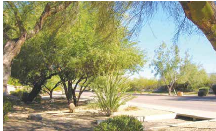
A sidewalk scupper diverts stormwater runoff from the street to adjacent right-of-way land, reducing street flooding, cleaning stormwater and supporting native edible trees.
