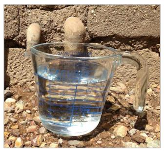
Using a measuring cup, this AC unit was determined to yield about 2 cups of water every five minutes on a humid August day. This equals around 36 gallons every 24 hours in these conditions.
